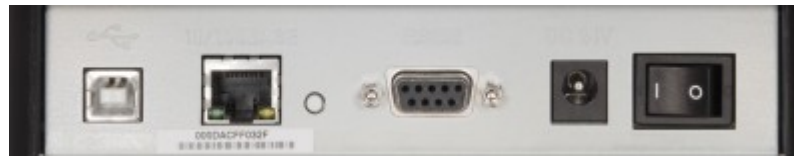
Featuring on-board LAN, USB and Serial interfaces.
